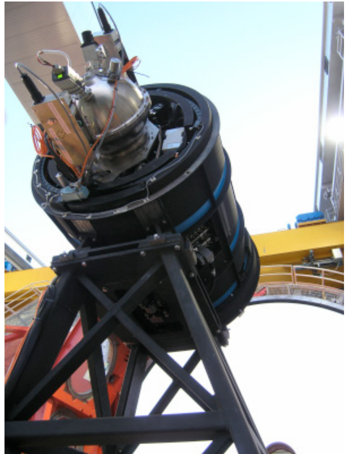
Fig. 1. The LBC-Blue instrument installed at the prime focus of the first LBT telescope unit.
