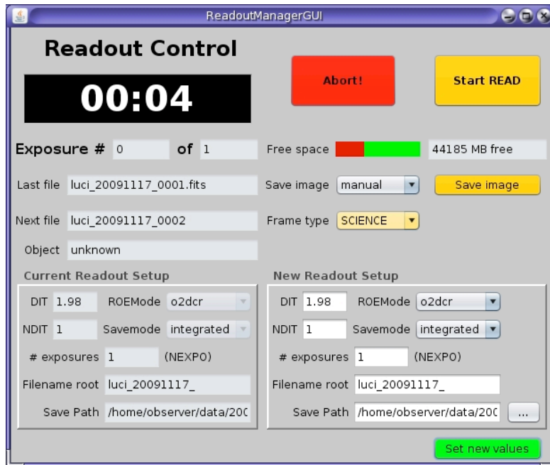
Figure 22: The LUCIFER Read Out Manager GUI. All necessary detector parameters can be set from this GUI.
