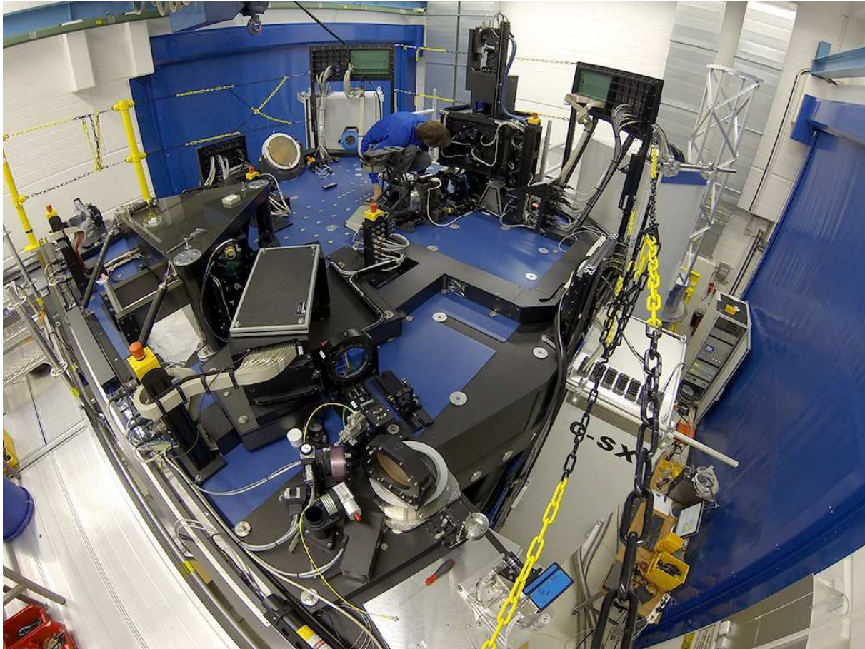
Figure 7. Picture in the integration hall at the MPIA in Heidelberg of the LN optical bench (reversed from left to right compared to Figure 6) showing recent progress in the assembly. Photo courtesy of Tom Herbst and the LN team.
