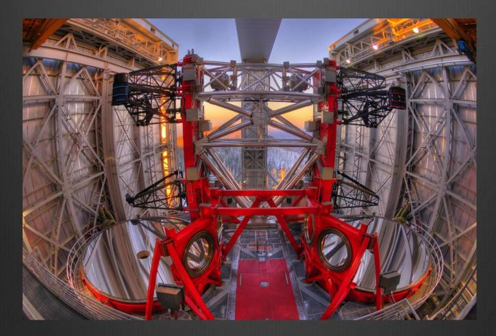
Two 8.4-m mirrors on the same mount – future interferometry Now: Two large telescopes with complementary instruments
