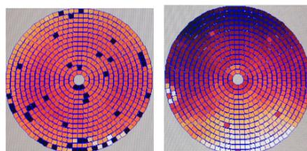
Fig. 2: Left: Example of current actuator positions with relative position color coding. Right: Actuator commands in terms of position, which qualitatively shows what the wavefront aberration looks like. Note the sprinkling of deactivated actuators in both images.
