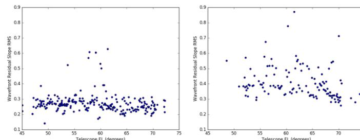
Fig. 5: Wavefront slope RMS residuals at different elevations during the night of April 5, 2017. Lower elevations produce poorer correction, and there are clear personality differences between the two sides.
