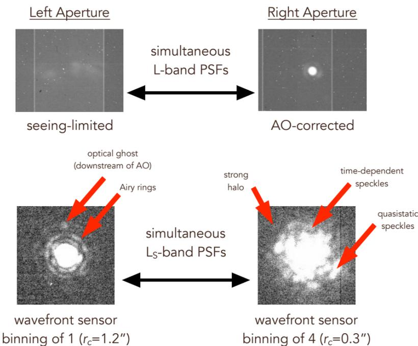
Fig. 3 (left): Top row: LMIRcam readouts showing the effect of AO. Bottom row: Variation in PSF quality depending on wavefront subaperture binning, with shade scaling to show the area outside the PSF cores.
