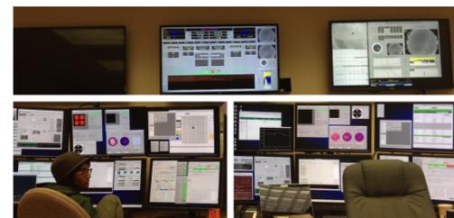
Fig. 6: The AO operational setup in the remote room in Tucson, AZ. This image is split into parts to indicate telescope and weather telemetry (top), left aperture AO operations (bottom left) and its right aperture counterpart (bottom right). All three parts are required to produce a double-sided AO correction, and require a two-person team.
