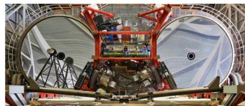
Fig. 1: View of the LBT primary mirrors, with LBTI inside the rectangle formed by the red trusses between the two apertures. (Credit: LBTO, Enrico Sacchetti)
